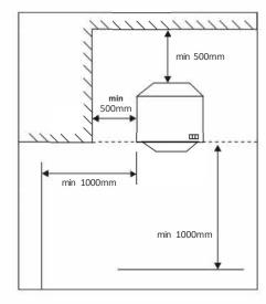
At MAX setting the Heater requires a MINIMUM of 52.5 Sq Cm of ventilation both at a high and low level within the room, YOUR HEATER CONSUMES OXYGEN WHILE IT IS WORKING. FOR THAT REASON ADEQUATE VENTLATION SHOULD BE PROVIDED IN ROOMS IN WHICH THE HEATERS IS USED. THIS ENSURES THE REMOVAL OF PRODUCTS OF COMBUSTION AND ALLOWS THE ENTRY OF REPLACEMENT AIR.
