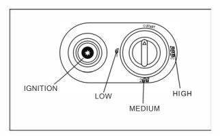
**Note:** On first lighting a heater from new or after a period of non use, it may be necessary to hold the control knob down for a longer time than stated above in order to allow gas to flow to the pilot and purge air from the system.
